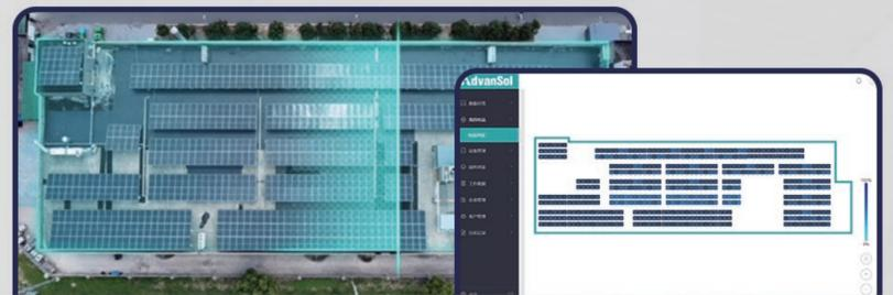
The MR series not only has a module-level rapid shutdown function, meeting the safety requirements of the US NEC 690.12-2014, 2017 and 2020 for photovoltaics, but also can monitor the power, voltage, current and other parameters of any panel in real time, and collect and upload them to the Acloud platform through the data controller (V2.5 data control box).
